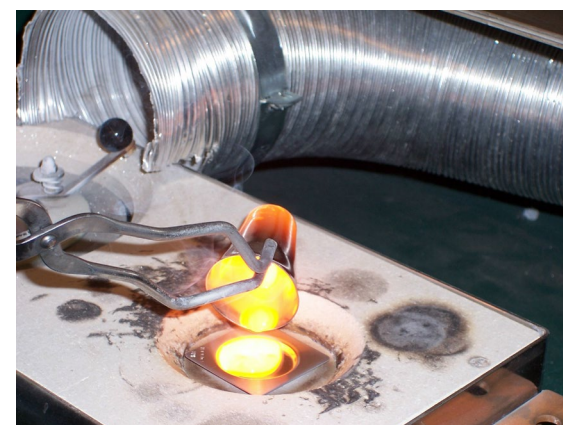
Texts of waste material being exposed to right temperature (800°C) in a special oven cooperation with the Institute of Applied Geosciences and the Geochemical Laboratory, TU Berlin
